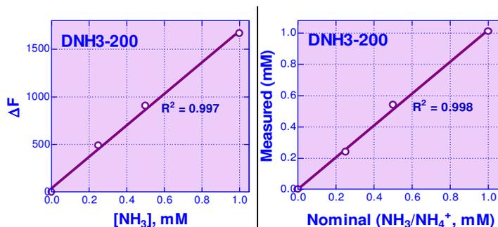
Left: standard curve performed on a 96-well plate reader (Spectramax M2);
